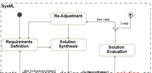
Based on predefined requirements, the system designer builds a solution on system synthesis. The acceptance of -a -certain -solution- depends on -the evaluation process, which is performed through requirements verification.
